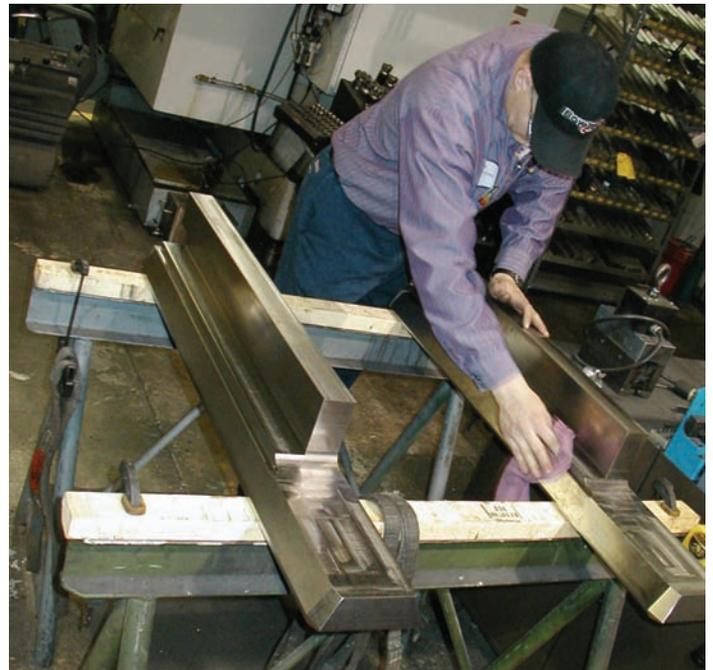
Jed Millikan, Norfolk Specialties, cleans these "clamp bars" after plunge roughing and finishing surfaces on a Milltronics RH30. Plunge roughing removed 278 pounds from the 665-pound, 4140 pre-hardened billet. Eight more operations – including drilling, boring, counterboring, countersinking and tapping holes at various angles – remove an additional 60 pounds, resulting in a finished component that weighs half as much as the raw stock.
