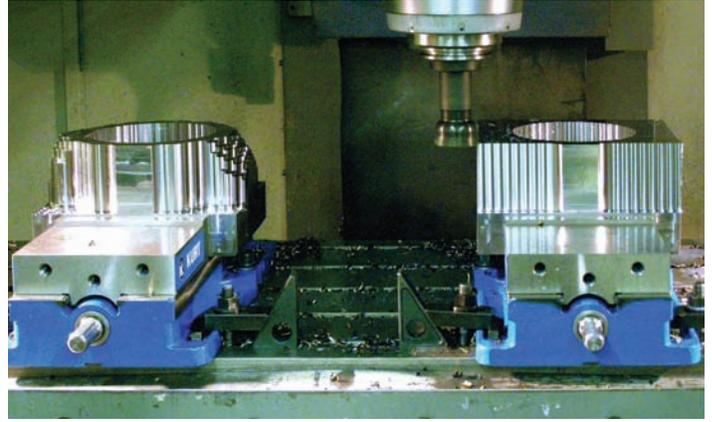
A 2.5" Sandvik plunge mill roughs stock for a pair of Ouvreson steering knuckles. The 18-pound final part is machined from a 190-pound block of 1018 plate steel. GibbsCAM Plunge Rough reduced roughing time from 1.75 hours to 45 minutes.
