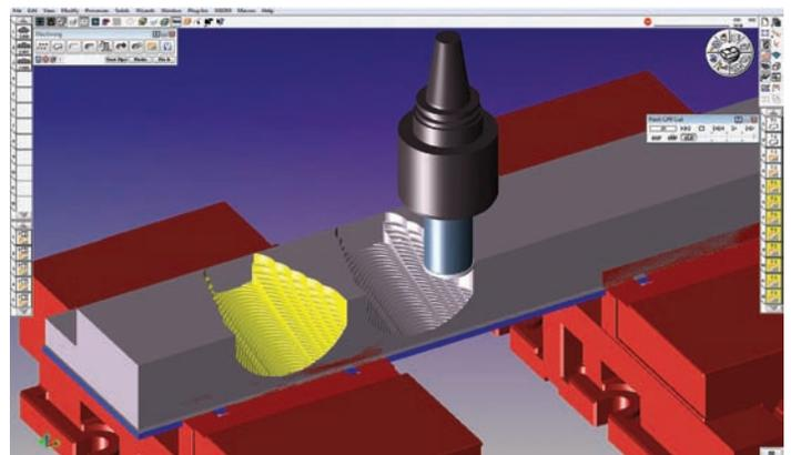
At Norfolk, GibbsCAM's plunge roughing routine has cut on-machine time in half and quadrupled tool life.
